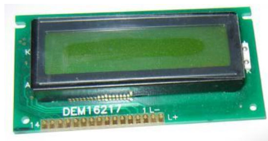
Figure 1: A typical LCD module.
